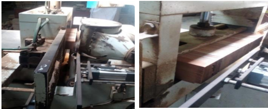
Figure 2: Finger cutting machines
